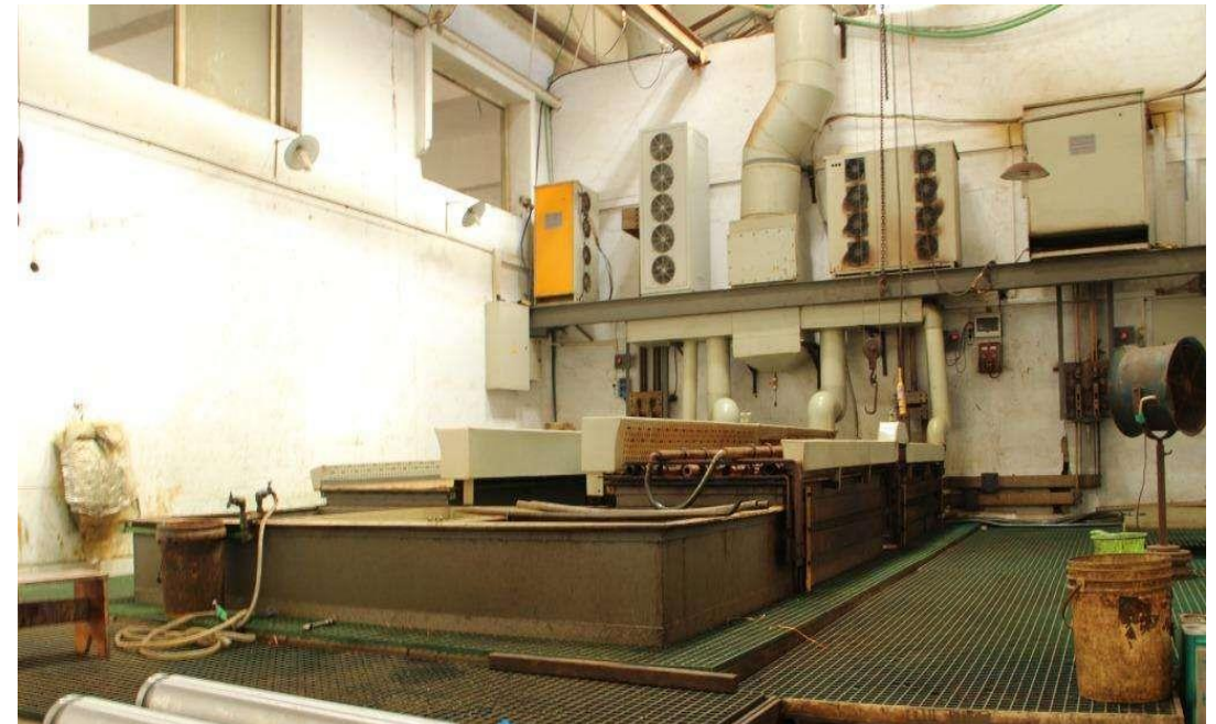
Fig.2 Hexavalent chromium plating line in China
